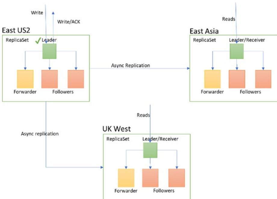
Figure 6-9. Write acknowledgment (checkmarks depict committed writes)
