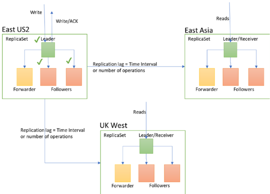
Figure 6-7. Write acknowledgment (checkmarks depict committed writes)
