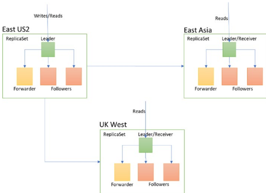
Figure 6-2. Database with ReplicaSet within geographical as well as cross-geographical regions
